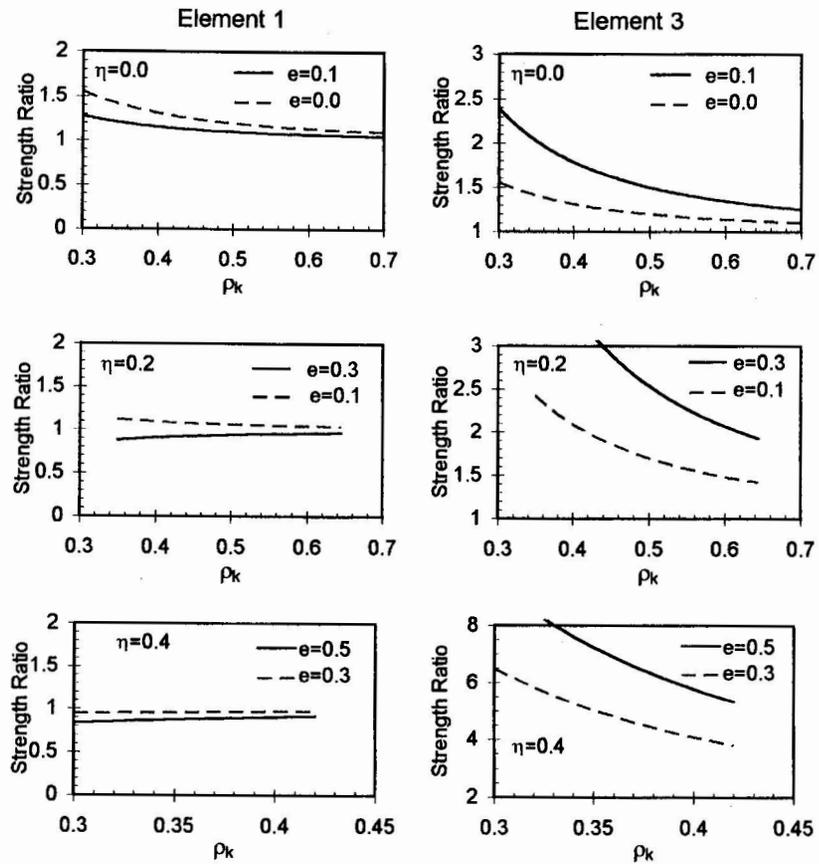
Fig. 2 Strength ratios of longitudinal edge elements
