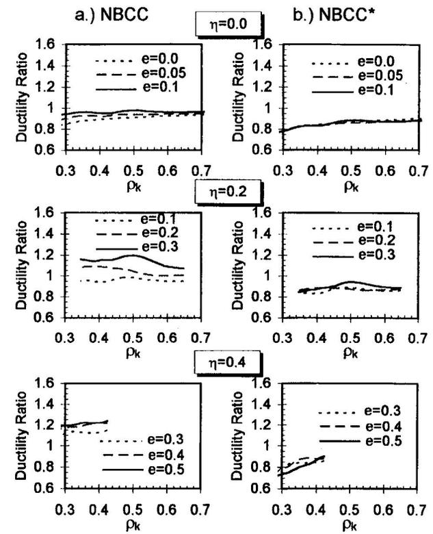
Fig. 5 Ductility ratios for element 4 for systems designed using a.) NBCC and b.) modified NBCC
