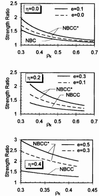
Fig. 3 Strength ratios of transverse edge elements
