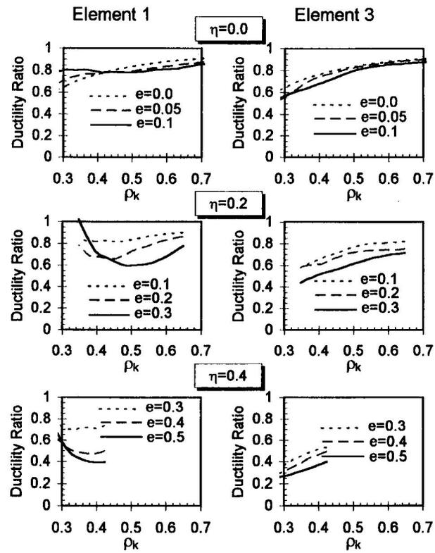
Fig. 4 Ductility ratios for elements 1 and 3 for systems designed using NBCC
